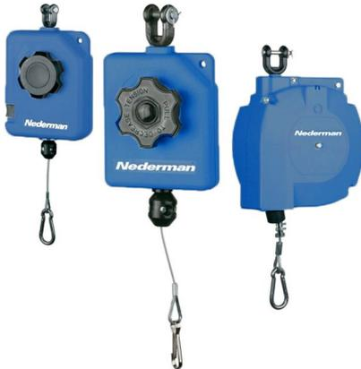
Series 810 balancer makes the tool weightless and minimizes the strain on the operator. The balancer comes in three different models and in nine weight classes, with a span from 0.5 kg to 10.9 kg (1 lb to 24 lb).
