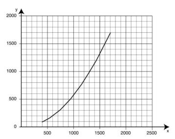
X: airflow, m³/h, Y: static pressure Pa
