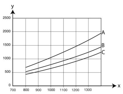
X: airflow, m³/h, Y: static pressure Pa,
