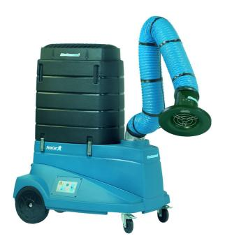
FilterCart W3 mobile filter unit for extraction in light production applications is "state of the art" with all possible features. Includes a warning signal when the filter is full. The W3 model fulfills the legislations W3 from BGIA. The specially designed metal hood with integrated spotlight creates maximum air velocity at the welding spot.
