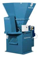
The integrated system crushes the chips, de-oils the chips and recovers coolant.
