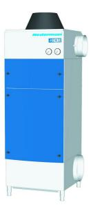
Designed for lathing and milling applications, for machines stamping and pressing steel plates, industrial washing machines, abrasive water jets etc. In all metal fabrication with oil mist troubles, these filters will fit into a ducting system, connected to each machine. All units are equipped with pres-sure gauge for control of filters as well as a indication for need of cleaning (self draining). Suitable for emulsions and neat oil.
