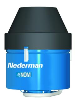
The NOM 4 is an oil mist filter in compact design and therefore suitable for enclosed cabinet single CNC machines. The unit is easy to install and enables maximum flexibility in the workshop, as it is normally installed on top of the machine. The NOM 4 is suitable for emulsions and pure oils.
